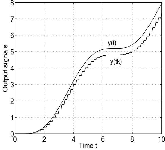
Fig. 3. Continuous and discrete open loop responses
