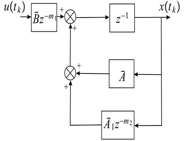
Fig. 2. Approximate discrete time system
