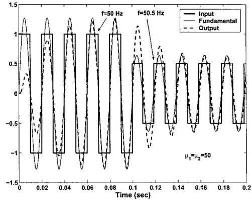
Figure 5. Somewhat unexpected adaptive feature of the APM filter is demonstrated in this figure. Slight variations in frequency are tracked by the filter.
