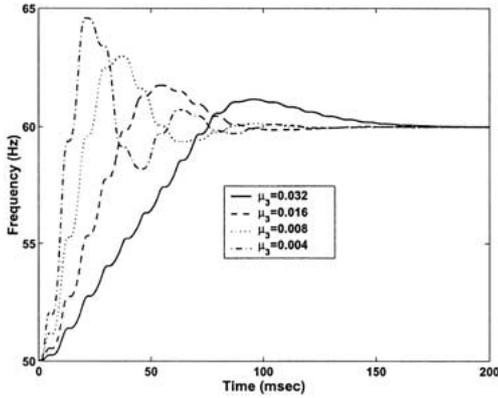
Figure 8. This figure verifies the effect of  $\mu_3$  on the performance of the APFM when is used as a frequency estimator. As expected by the Theorem 2, reducing  $\mu_3$  moves the system towards instability.
