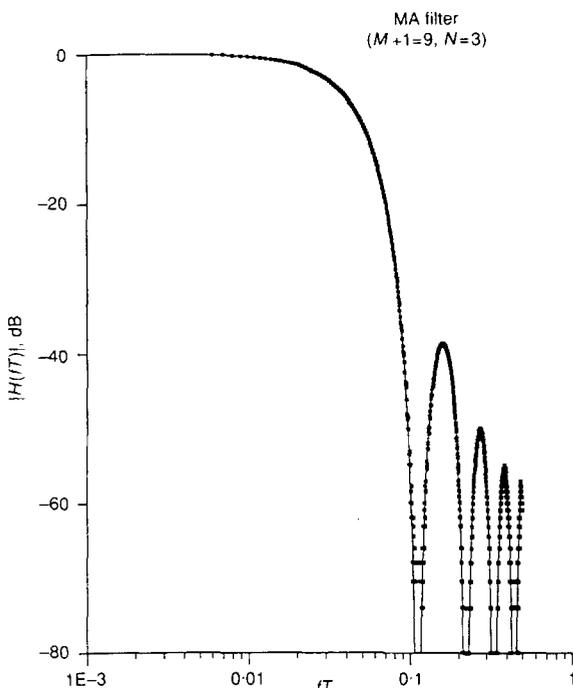
Fig. 3 Log magnitude of filter response ( $N = 3$ ,  $M = 8$ ): estimated response (■) from filtered sweep signal using cross-spectral techniques and theoretical response (solid line) from eqn. 2
