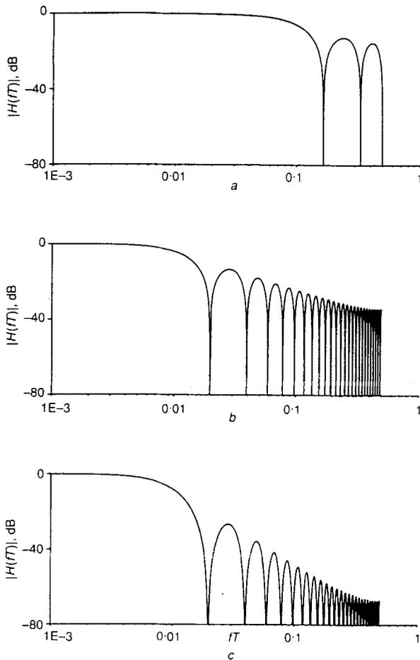
Fig. 1 Typical examples of the log-magnitude frequency responses of  $N$  times repeatedly applied  $M + 1$  unweighed moving average filter; (a)  $M = 5$ ,  $N = 1$ ; (b)  $M = 50$ ,  $N = 1$ ; (c)  $M = 50$ ,  $N = 2$
