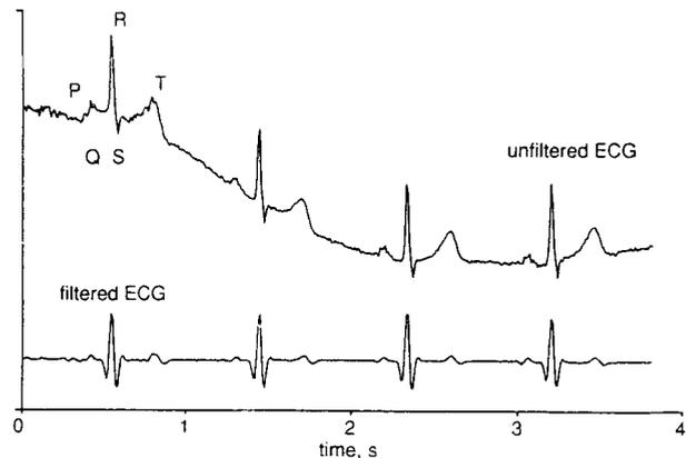
Fig. 4 Unfiltered and filtered electrocardiogram-recordings; dominant low-frequency drift phenomenon and T-waves, as well as high frequency noise and P-waves, effectively reduced by moving average filter: low-pass:  $N = 5$ ,  $M = 8$ ; high-pass:  $N = 1$ ,  $M = 66$
