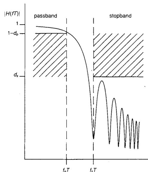
Fig. 2 Specification of low-pass filter by ripple  $d_p$  and edge  $f_p T$  of passband and ripple  $d_s$  and edge  $f_s T$  of stopband; solid line represents a possible realisation
